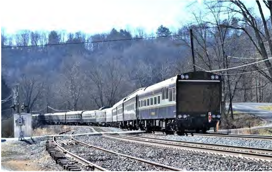
My last shot of P001-23. It is a rear view of W. Thomas Rice . Note the large glass window covering the rear of the car. Behind the window are three rows of theater seating. At night the lights above and below the window are used to illuminate the track for viewing.
