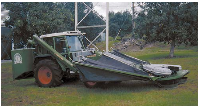
Figure 2.2. Tree shaker with padded jaws and canvas skirt (retracted) that normally catches the falling nuts.
