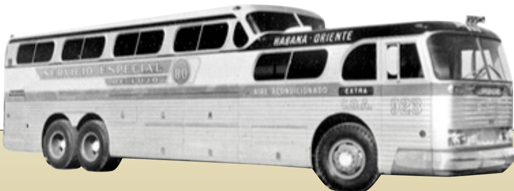
The split-level coach liners of the 1950s introduced long distance, luxury travel across the U.S. featuring characteristic scenic view windows. The 43-seater Beck DH with Cummins 300 hp HRBS-600 was one of the most powerful models built, with some exported to fleets in Cuba and Mexico.
