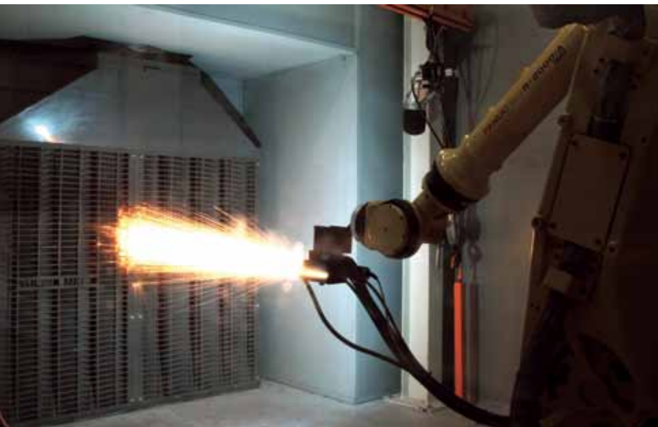
A robotic arm sprays metal onto a worn surface to facilitate remanufacturing.
