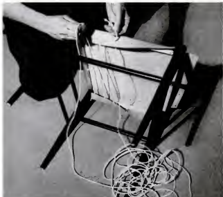
LEATHER SEAT (also the canvas variety) is laced to the frame with cord. This lacing is worked from the front to the back first, then from side to side.
