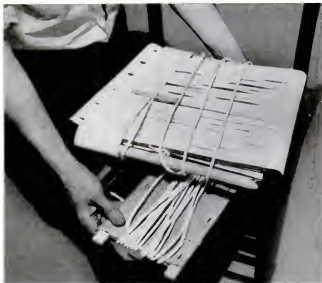
WINDING IN OTHER DIRECTION follows the side-winding (preceding page). Where lengths of rope join, glue is put on knot to prevent loosening.
