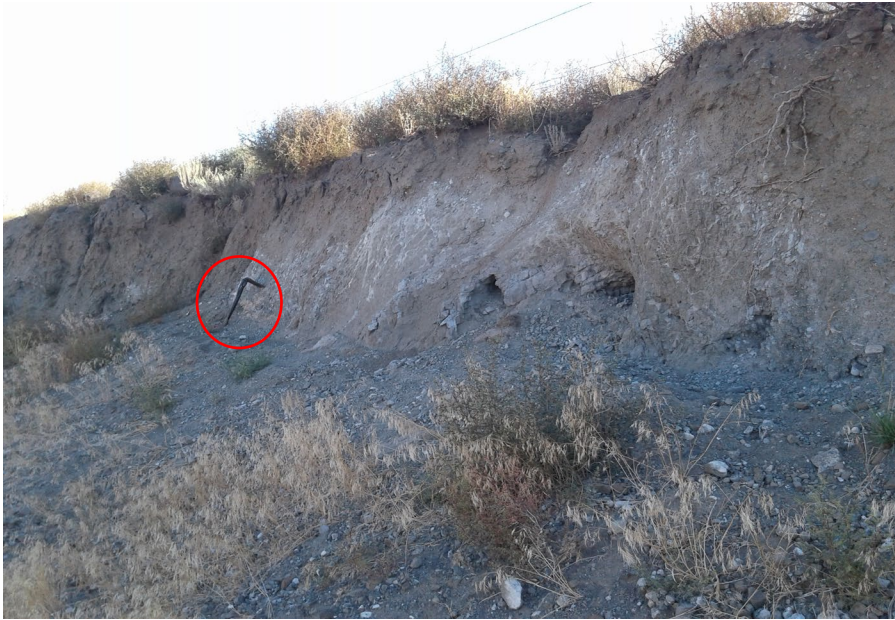
Figure 12. Soil formed in glacial till and loess visible in roadcut just north of intersection of roads 5 NE and S NE. Note the rocks throughout, and the poorly formed, white calcium carbonate accumulations (Bk horizon?). Poor soil development overall indicates relative youthfulness of soil. Note shovel (red circle) for scale. Author photo, 09/10/2023.
