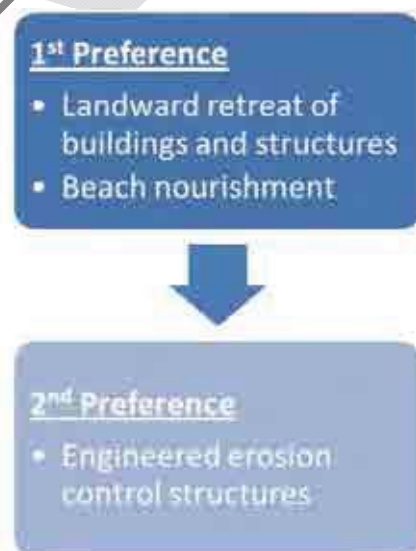
Figure 2-1 Hierarchy of Recommended Erosion Management Strategies for Buildings and Structures in the Erosion Prone Area
