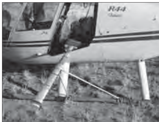
Helicopter mounted with distance-interval marked booms as used in aerial surveys for feral pigs.
