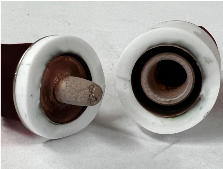
Figure 8c. Internals of spark gap following tests at 2500Arms. The sample failed open.
