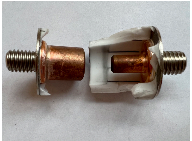
Figure 8d. Internals of the spark gap prior to testing
