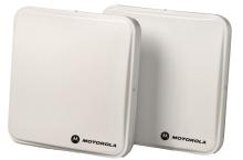
This all-purpose antenna can be used in standard RFID applications with power levels up to one watt, as well as custom high-power applications requiring up to 20 watts. The antenna is traditionally used in pairs, with right and left hand polarization.
