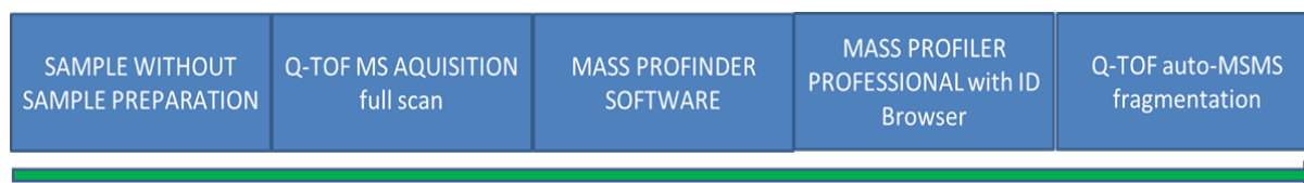
Figure 158: Non-target workflow used for analyses by UHPLC-Q-TOF-MS
