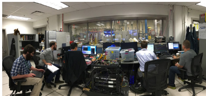
University of Colorado and AFRL teams in the control room during the dual-mode ramjet ground test. The modified dual frequency comb system is in the center foreground, and is sending light to the test cell, which is located beyond the control room windows.
