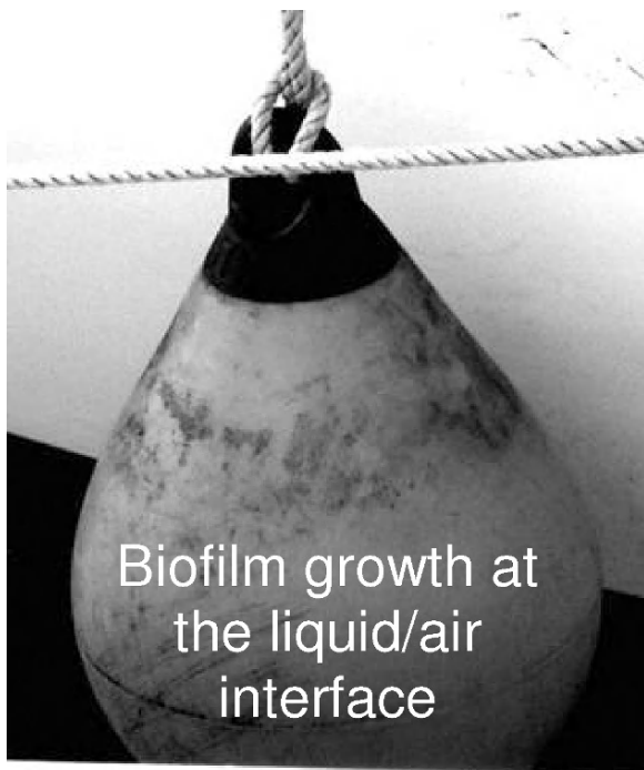
Fig. 1 Plastic buoy that has biofilm growing on its surface, resulting in fouling of the material
