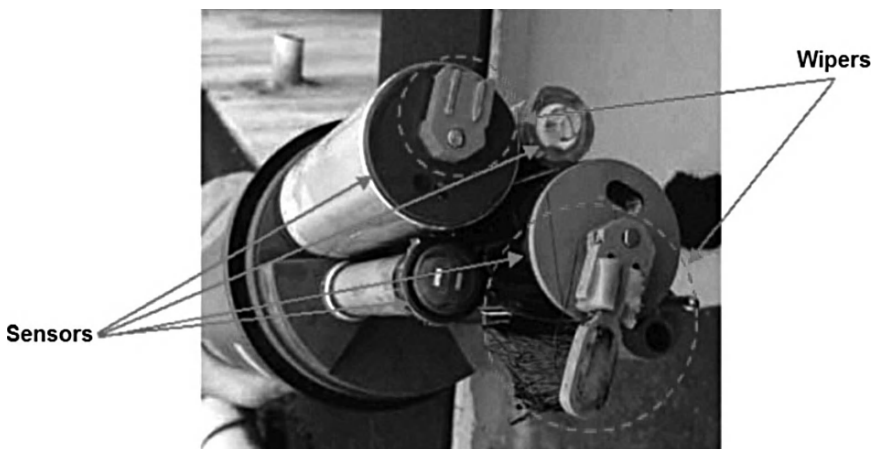
Fig. 5 Multiparameter probe with a mechanical biofouling protection based on wipers (photo: L. Delauney, Ifremer, France)
