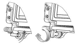
6. Tighten the keyboard tray locking knobs to secure the tray in position.
