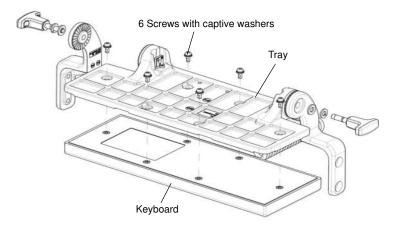
Attach the left and right mounting arms to both sides of the VC70, using the M5x14mm Torx head screws with flat and lock washers. Only tighten the cap screws three turns.
