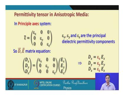
So, in such a principal axes system we can write the epsilon permittivity tensor as epsilon x x, epsilon y y and epsilon z z. If we if we represent with a sort notation then we can write that this is because there is no other components no other cross components x y, y z or z x. So, we can write that epsilon tensor as epsilon x, epsilon y and epsilon z.
