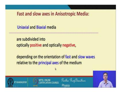
There are some more things so Uniaxial and Biaxial media are against subdivided into positive and negative optically active media depending on the orientation of the fast and slow waves. So, in some medium the one which is fast waves, in some other medium the same will be referred to as a slow waves. So, this is all relative to the principle axes system of the medium.
