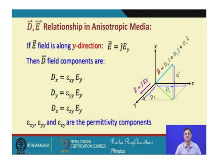
Next, let us consider the behavior when we apply an electric field along the y axis. In the same way the displacement vector will be in general not in the direction of the electric field, but in a in a direction which is different from the direction of the electric field. As a result, in the same way we can write the displacement vector in this case, the x component is equal to epsilon x y E y, for the y component it is epsilon y y E y, and for the z components it is epsilon z y E y.
