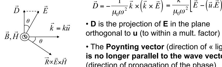
$$\vec{D} = -\frac{1}{\mu_0 \omega^2} \vec{k} \times \left(\vec{k} \times \vec{E}\right) = \frac{k^2}{\mu_0 \omega^2} \left[\vec{E} - \left(\vec{u} \cdot \vec{E}\right) \vec{u}\right]$$
