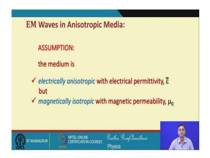
So, in the case of a general anisotropic medium in this discussion we will first make these assumptions that; the medium is electrically isotropic with electrical permittivity given by this epsilon bar that is a tensor, but the medium is magnetically isotropic with magnetic permeability, mu naught which is the free space permeability.
