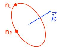
The polarization directions that have a max and min index of refraction form the major and minor axes of an ellipse defining  $n(\theta)$  the index fora wave with the electric displacement vector at an angle of  $\theta$  in the transverse plane.
