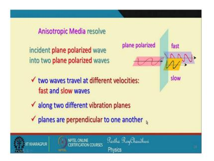
So, in anisotropic medium, incident plane polarized light will decompose into 2 plane polarized light. So, let us suppose that you have an incident plane polarized light this will immerge out from the medium or within the medium, within the medium in 2 mutually orthogonal directions. And in general the 2 waves travel at different velocities these are; the one which is faster will be called the fast waves, and the one which is slower will be the slow waves.
