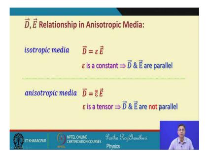
So, looking at the E D relationship in anisotropic medium the constitutive relation in this case is, the displacement vector is equal to the epsilon times the electric field vector, which is for isotropic medium this epsilon is a constant. And as a result it is a scalar being and the D and E are parallel. So, the electric field vector and the displacement vectors will point along the same direction where as in the case of anisotropic media this D and E in general are in different directions.
