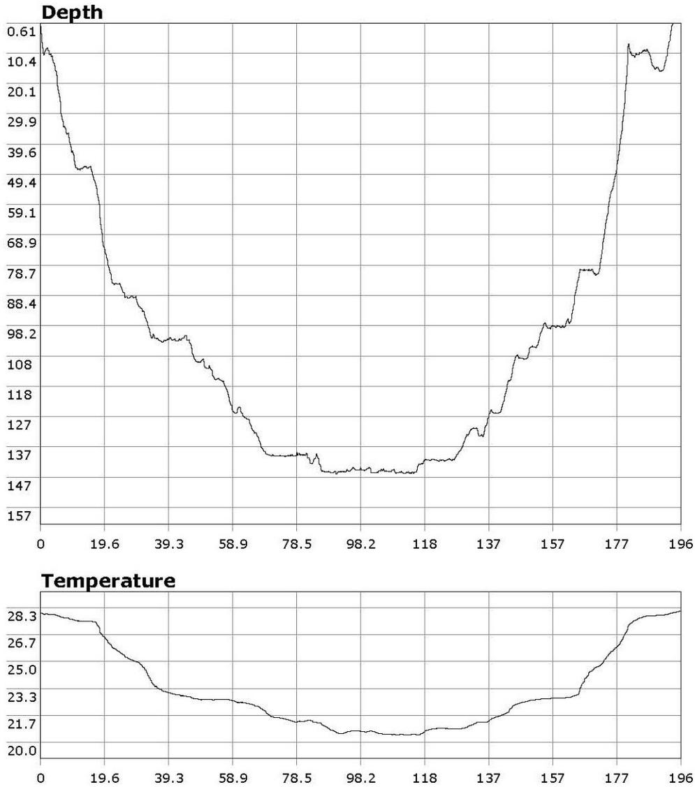
Kralendijk Pier (DIVE 1) depth (m) and temperature (°C) profile (x-axis in minutes of submersible dive time)
