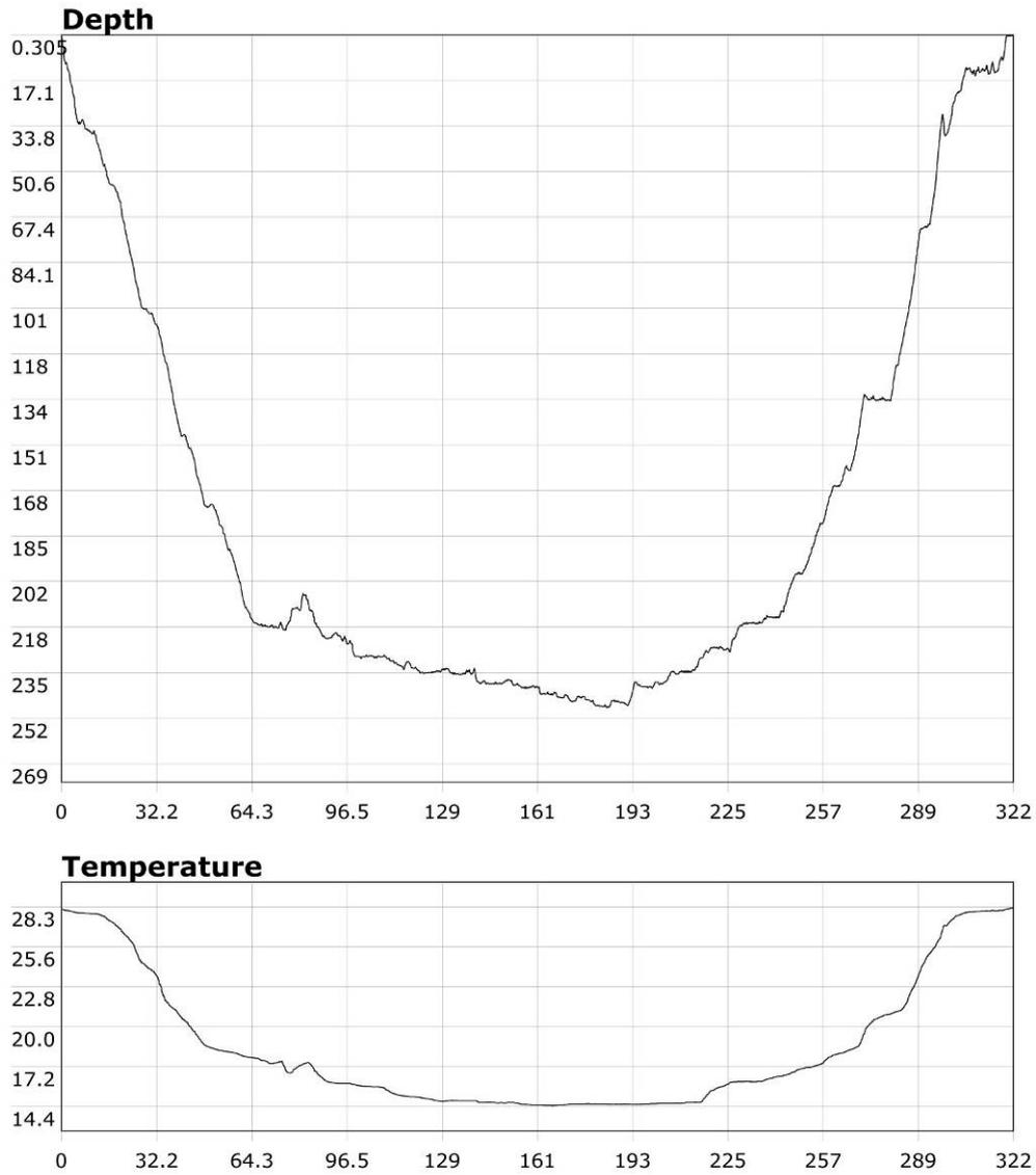
Cargill pier (DIVE 3): depth (m.) & temperature (°C) profile (x-axis in minutes)
