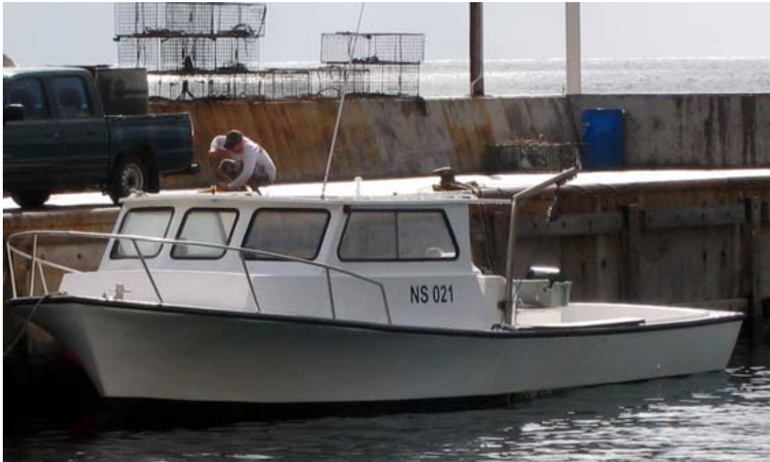
Figure 15. A typical commercial fishing vessel used for trap fishing on Saba Bank. Note the davit and hydraulic wench mounted to port side behind the wheelhouse.
