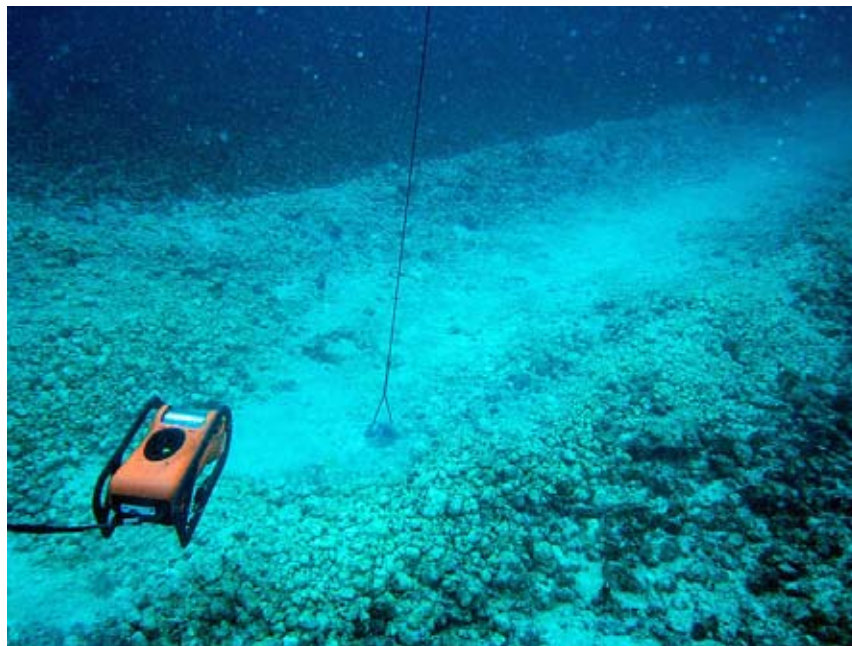
Figure 22. Remotely operated vehicle exploring an anchor scar. (source S. Lundvall)
