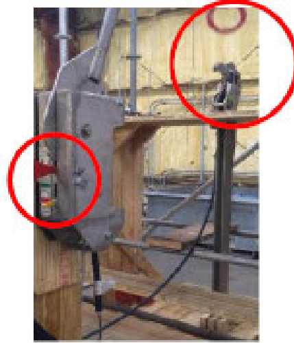
Image 53: If the locking shaft turns enough, the hook will release, even as the release handle stays locked.
