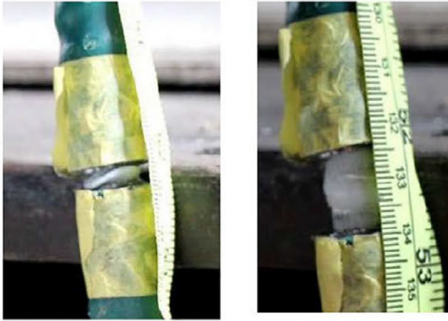
Figure 60 (far left) and 61 (right): The white polyethylene liner evidencing forces of compression and stretching after the wire layer is fully compromised. These photos were taken during the Coast Guard's experiment at MSTC. Credit: CG.
