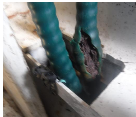
Image 6: Photograph of damage to Lifeboat No. 6 aft control cable dated June 6, 2019. Credit: Palfinger.
