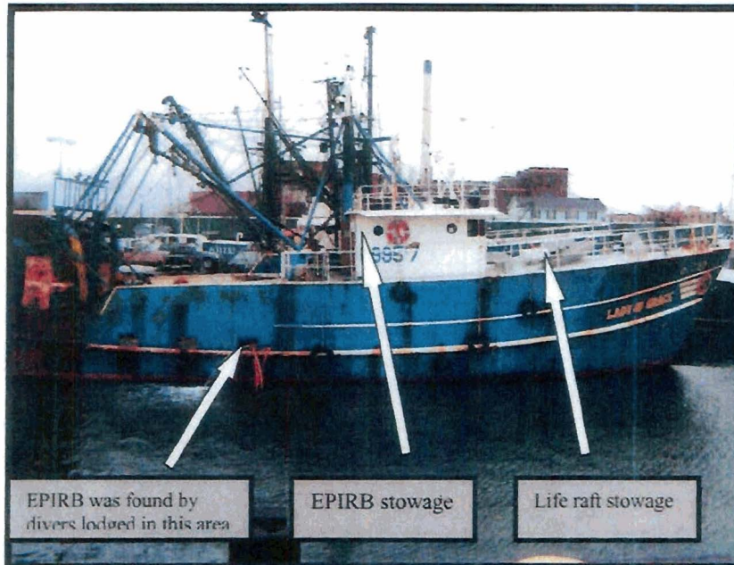
Photo 5: Storage locations of EPIRB and Liferaft
