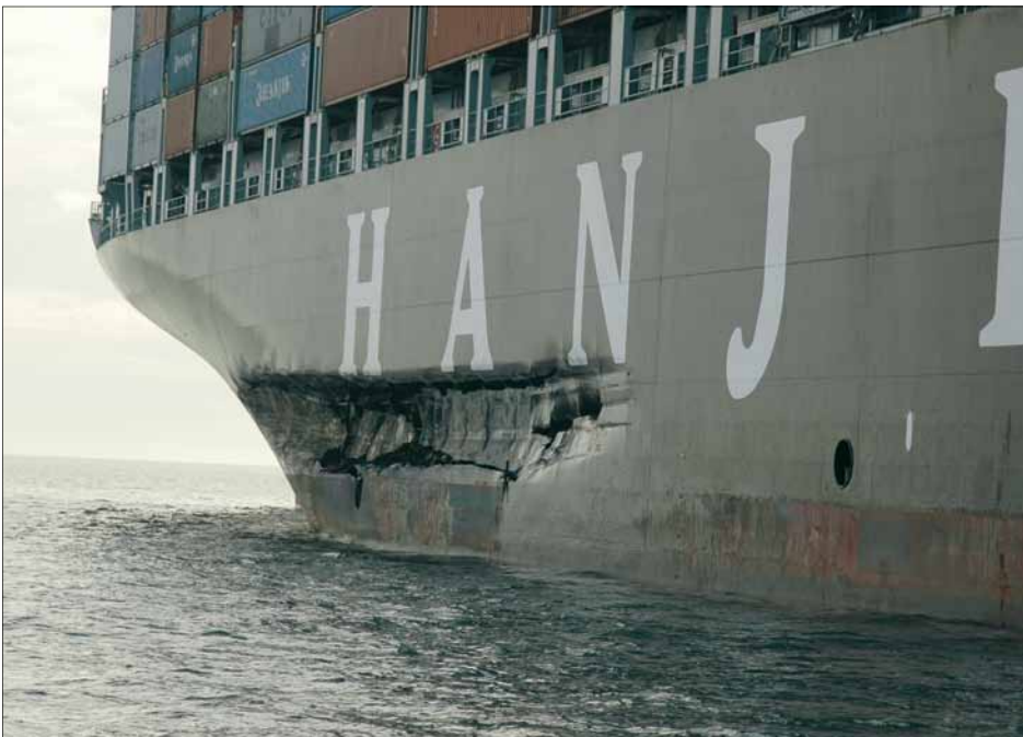
Above is damage to the 900-foot container ship Cosco Busan . The damage occurred after the cargo ship hit the San Francisco Bay bridge, spilling bunker fuel into the San Francisco Bay. U.S. Coast Guard photo by Petty Officer Melissa Hauck.
