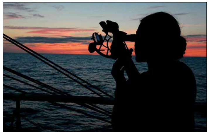
A Coast Guard watchstander uses a sextant to get a celestial fix. Some navigation principles are largely unchanged between military and commercial vessels.
