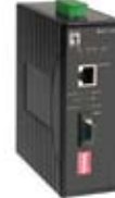
IEC-1840 RJ45 to SC Fast Ethernet Industrial Media Converter, Single-Mode Fiber, 40km, -40°C to 75°C, IEC61850
