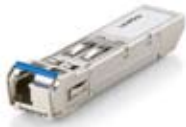
SFP-4310 1.25Gbps Single-mode BIDI Industrial SFP Transceiver, 10km, TX 1310nm / RX 1550nm, -40°C to 85°C
