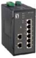
IES-0852 8-Port Web Smart Fast Ethernet PoE Industrial Switch, 802.3at PoE+, 4 PoE Outputs, 120W, -40°C to 85°C
