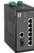
IES-0822 8-Port Fast Ethernet PoE Industrial Switch, 802.3af PoE, 4 PoE Outputs, 1 x SC Multi-Mode Fiber, 61.6W, -40°C to 85°C
