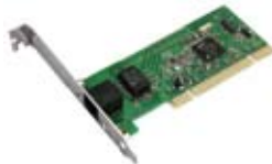
GNC-0105T Gigabit PCI Network Card
