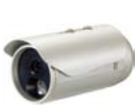
FCS-5053 Fixed Outdoor Network Camera, 3-Megapixel, 802.3af PoE, IR LEDs
