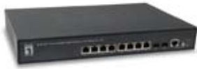
GEP-1061 10-Port L2 Managed Gigabit PoE Switch, 2 x SFP, 802.3at PoE+, 125W
