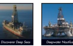
Transocean holds 19 of the past 23 world records for drilling in the deepest waters. Our ultra-deepwater drillship *Discoverer Deep Seas* set the current world water-depth drilling record in 10,011 feet (3,051 meters) of water in the U.S. Gulf of Mexico working for Chevron.
