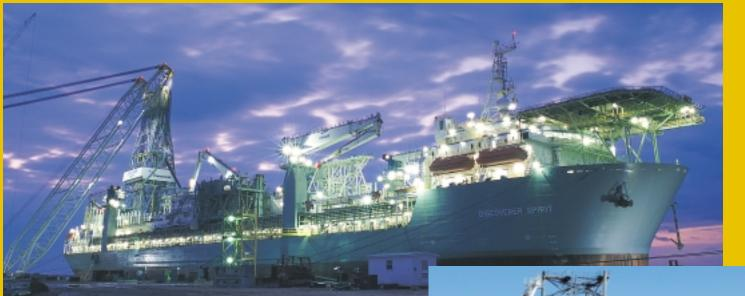
The setting of the dual-activity derrick on the ultra-deepwater drillship Discoverer Spirit in February, marks a milestone in the final stages of construction of the rig at the Aker Gulf Maritime shipyard near Corpus Christi, Texas, USA. Unlike the Discoverer Enterprise, which had its derrick set on the rig in three sections, AGM moved the whole derrick in one piece onto the deck of the Discoverer Spirit.
