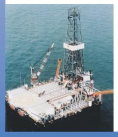
n the U.S. Gulf of Mexico, the *Transocean Marianas* has extended its string of world records for deepwater drilling by a moored semisubmersible. After setting three world deepwater mooring records last year, the upgraded high-specification semisubmersible set another milestone in January 2000 by drilling in 7,529 feet of water using a mooring system with suctionanchor technology.
