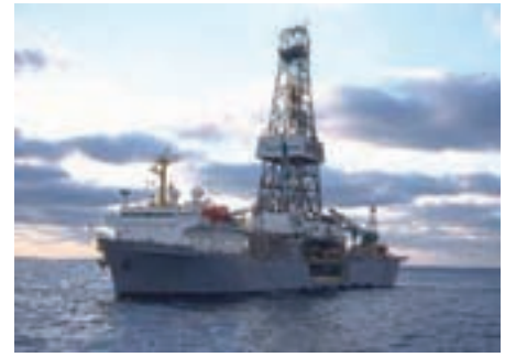
The Discoverer Seven Seas drillship is drilling exploration wells in deep water for ONGC offshore India's east coast.
