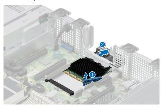
Figure 23. Removing the OCP Card in R760xs
