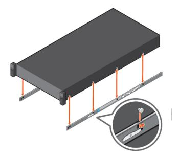
Figure 38. Attach the inner rails to the system
