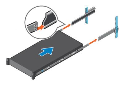
Figure 39. Install system into the extended rails
