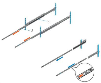
Figure 37. Pull out the intermediate rail
