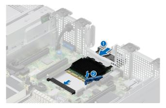
Figure 22. Installing the OCP Card in R760xs
