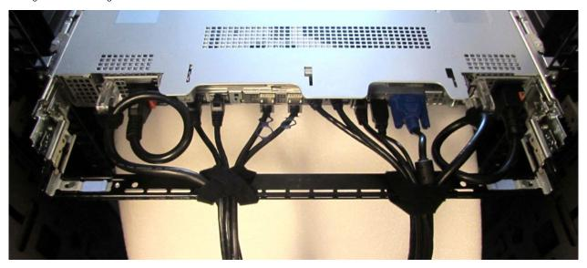
Figure 33. Cabled strain relief bar
