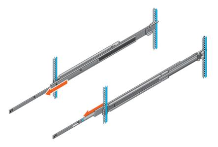
Figure 34. Pull out inner rail
