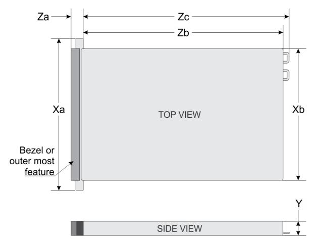
Figure 41. Chassis dimensions
