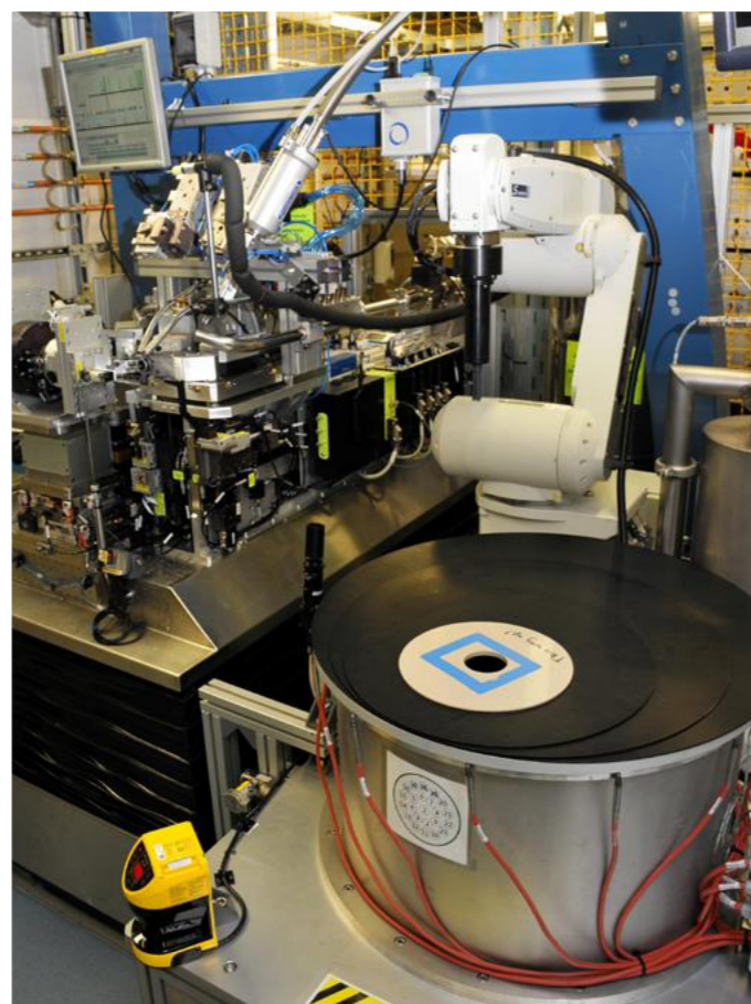
FIGURE 2: Robot used for automated protein crystallography at the Diamond Light Source. Source: https://www.diamond.ac.uk/industry/Industry-News/Latest-News/Synchrotron-Industry-News--MXnews4/MX-Sample-changer-upgrade-BART-.html
