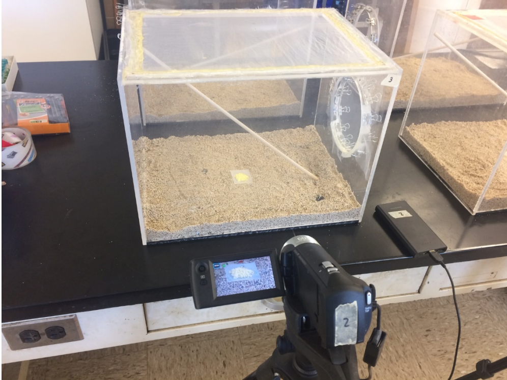
Figure 2-1. Example of cage used to test attraction of picture-winged flies to Amdro Ant Block bait. A small pile of Amdro bait, placed on a piece of plastic, sits in the center of the cage. At bottom of image is a video camera, zoomed in on the Amdro bait, used to film potential fly visitation to bait. Control cages were identical except no Amdro Ant Block bait was provided.
