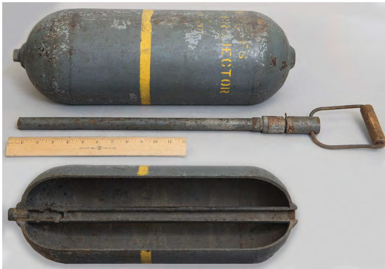
Figure 181: Mortar, 8-inch, Livens Projector, MI, MII, MIIA1 - Photograph - Top: Intact, Bottom: Cutaway
