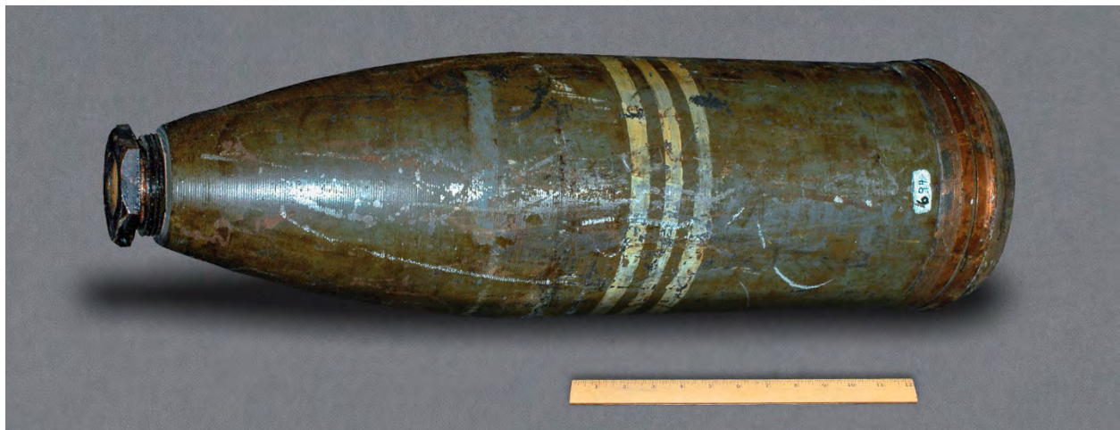
Figure 217: Projectile, 8-inch, Common Steel, Howitzer and Gun, MK III - Photograph
