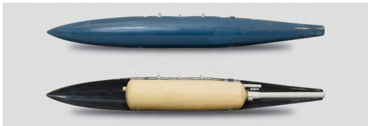
Figure 164: Tank, 84-gallon, Aircraft, Aero 14B - Photograph - Top: Model, Exterior, Bottom: Model, Cutaway View with simulated agent
