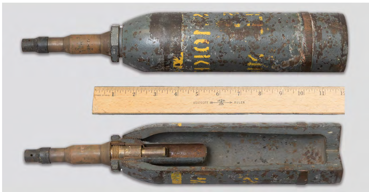
Figure 183: Projectile, 75-mm, MK II - Photograph - Top: Intact, Bottom: Cutaway View
