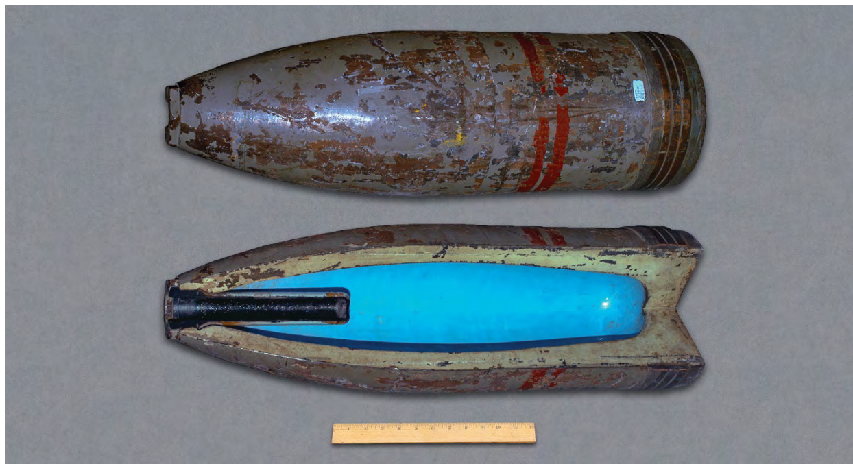
Figure 223: Projectile, 9.2-inch, MKI - Photograph - Top: Intact, Bottom: Cutaway View
