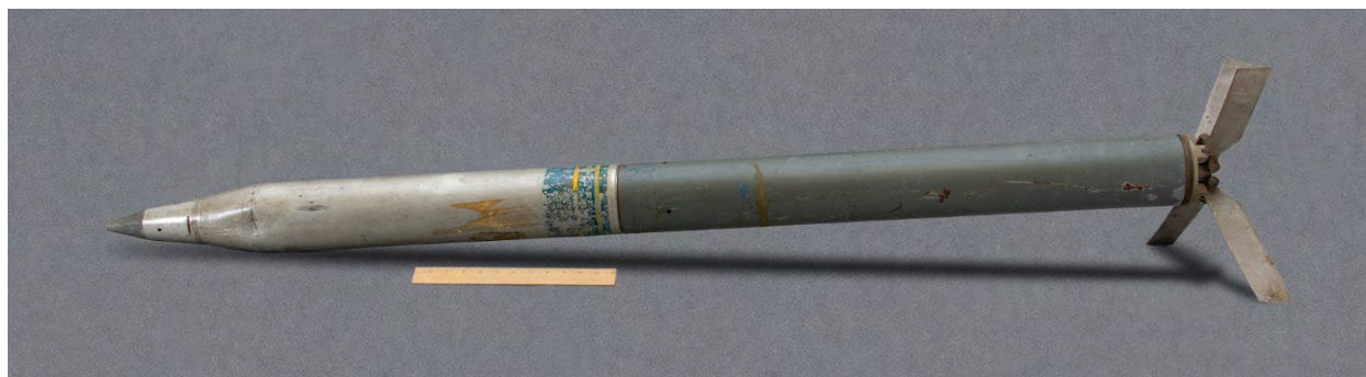
Figure 238: Rocket, 115-mm, Dummy Training, M60 (E49) - Photograph
