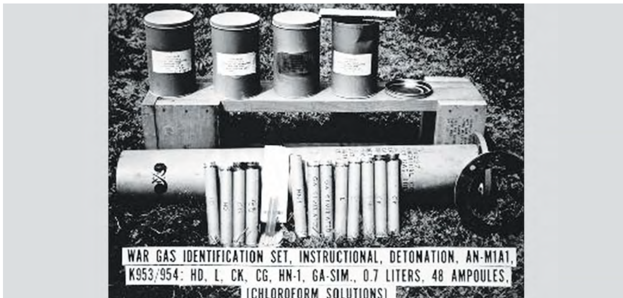
Figure 112: CAIS, War Gas Identification Set, Instructional, Detonation, K953/K954, AN-M1A1 - Photograph
