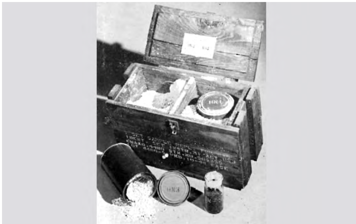
Figure 100: CAIS Replacement Set, Gas Identification, Instructional, Navy X Replacement Sets - Photograph
