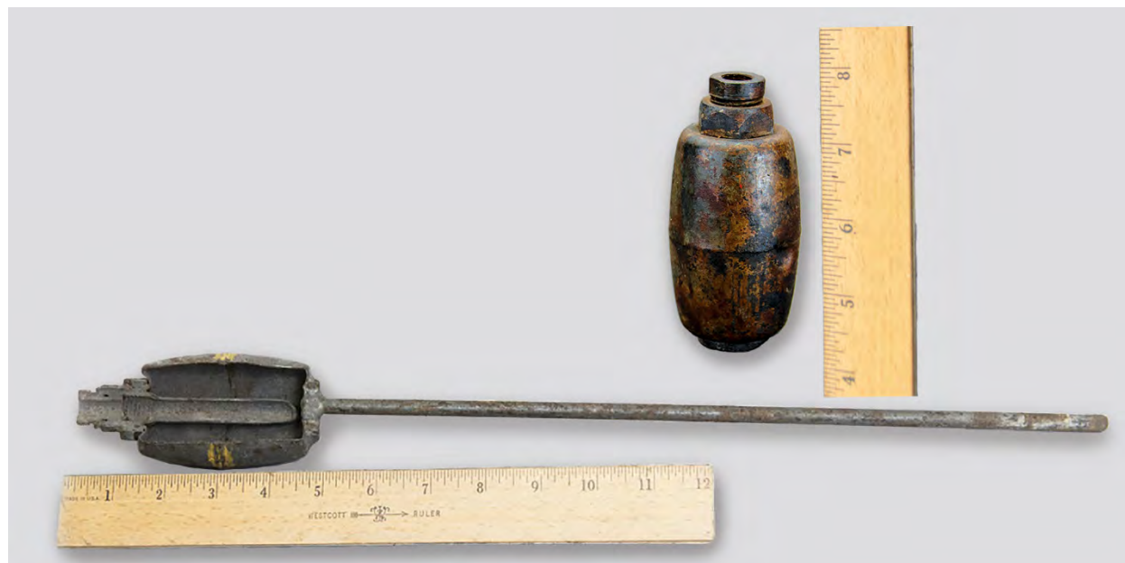
Figure 116: Grenade, Hand, MK1 - Photograph - Top: Intact, Bottom: Cutaway Rifle Projected, without Fuze (note the long rod attached to the base is part of the grenade as designed)
