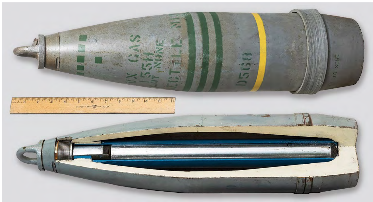
Figure 209: Projectile, 155-mm, Howitzer, M121 - Photograph - Top: Intact (Note: lug inserted), Bottom: Cutaway View
