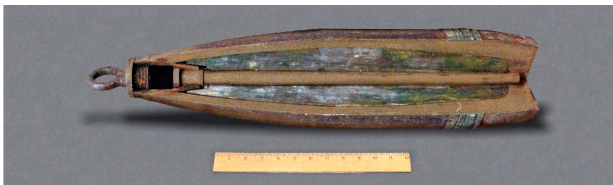
Figure 207: Projectile, 155-mm, Gun or Howitzer, M110 – Photograph - Cutaway
