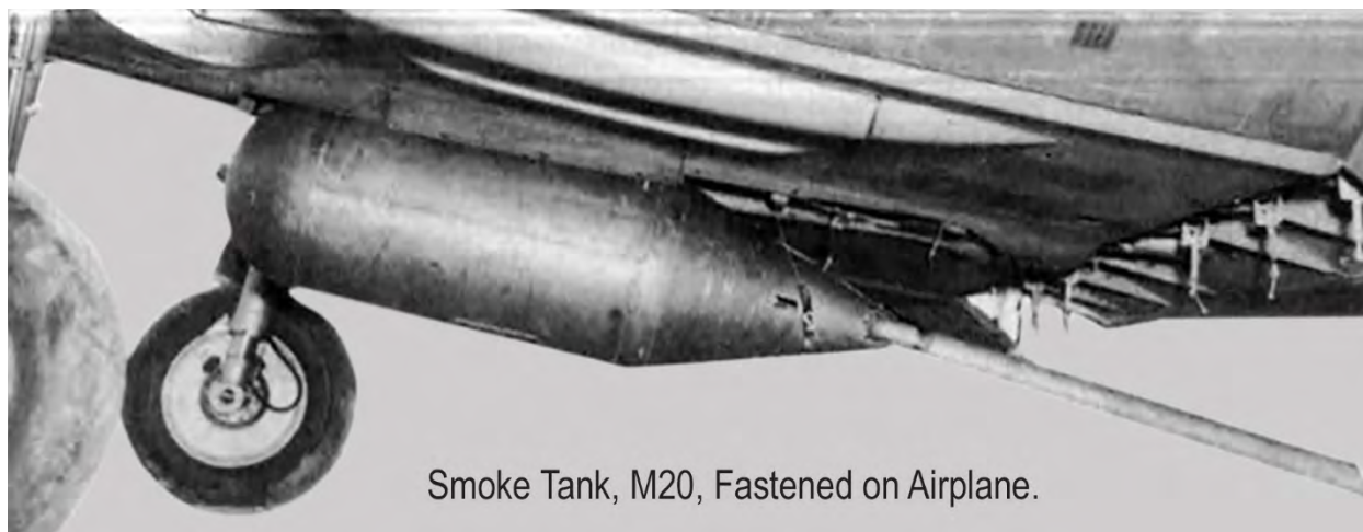
Figure 159: Tank, Airplane, 50-gallon, M20, Pressure – Photograph, Attached to Aircraft
