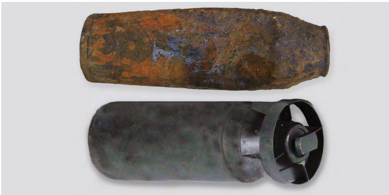
Figure 65: Bomblet, 10-pound, E49 - Photograph Top: Recovered, Bottom: Intact
