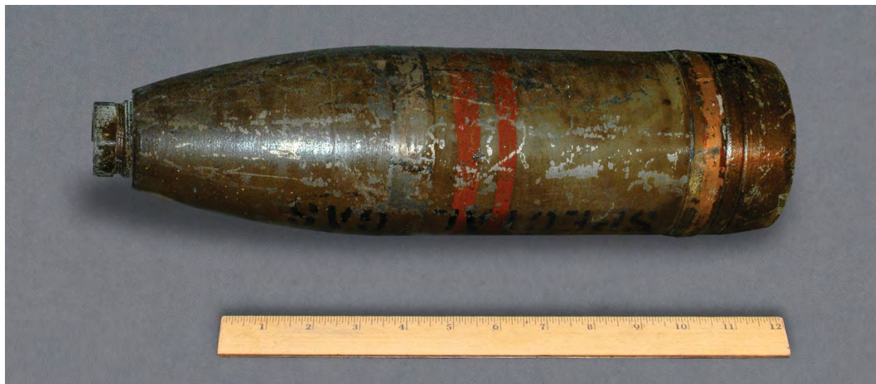
Figure 191: Projectile, 4.7-inch, Common Steel, MK II - Photograph
