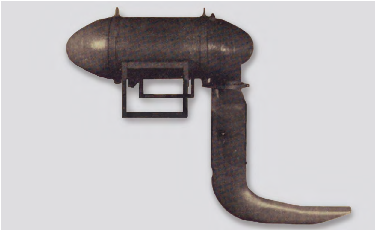
Figure 161: Tank, 70-gallon, Airplane, M33 and AN-M33A1 – Photograph
