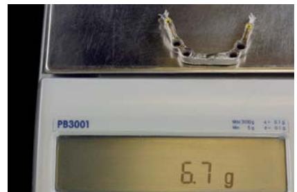
Figure 31. Bar construction with balance.
