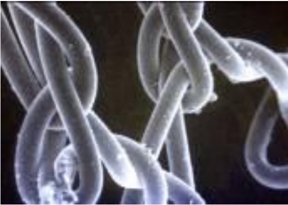
Figure 3. Mesh of plasma-filter SEM x60
