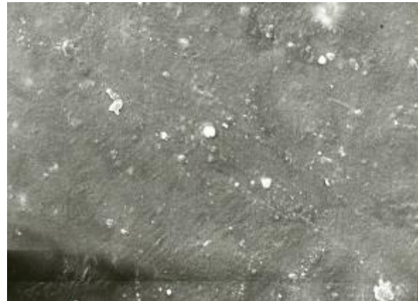
Figure 4. Surface of BIOPOL plastic not exposed to microbial degradation
