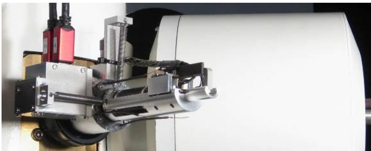
Figure 3. The high precision phase plate positioning device installed in a Zeiss LEO 922
