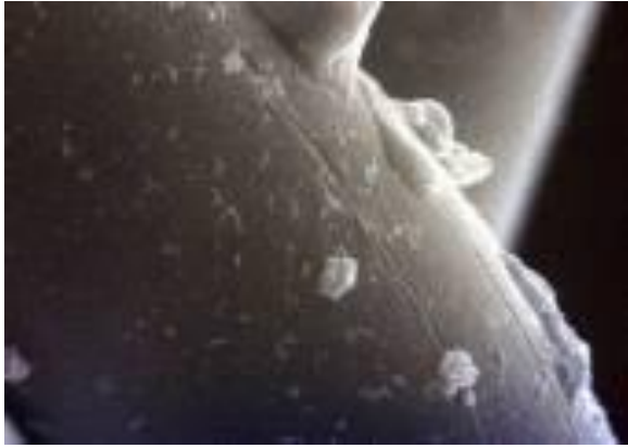
Figure 2. Catcher-mesh with single discrete particles SEM x1000
