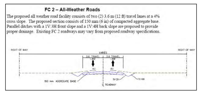
Figure C-4. FC-2 All-Weather Road (Diagram)
