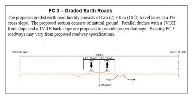
Figure C-6. FC-3 Graded Road (Diagram)
