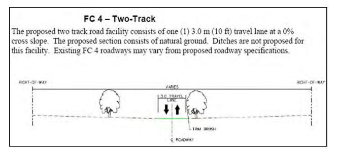
Figure C-8. FC-4 Two-Track Road (Diagram)
