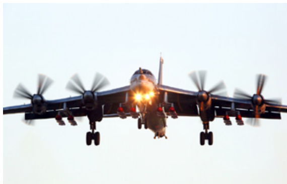
Kh-101/102 air-launched cruise missiles on a Tu-95MS heavy bomber; Moscow first used its precision strike arsenal in combat during a series of 2015 strike operations by sea- and air-launched cruise missiles against targets in Syria.
