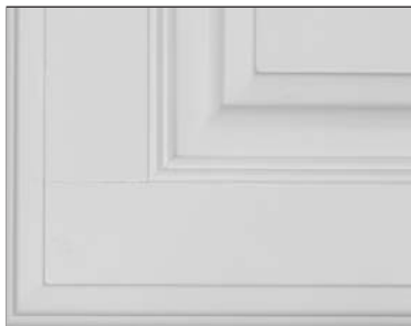
Example of front joint separation
