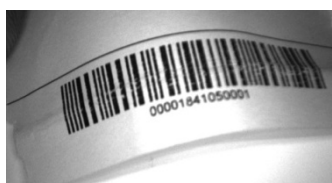
Figure 24 - Barcode Printed on Curved Surface Readable by Matrix 300N in spite of Image Optical Distortion
