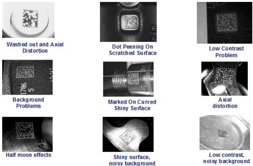
Figure 84 - Problematic Direct Part Marking Examples
