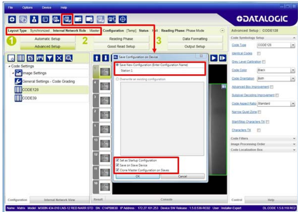
Figure 87 - Saving Synchronized Phase Mode Configuration to Master
