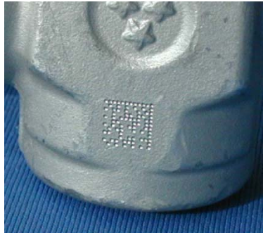
Figure 25 - Dot Matrix Code Directly Marked on Metal Surface by Using Dot Peening Technology
