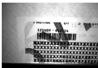
Figure 23 - Overprinted Barcode Readable by Matrix 210N also Through the Envelope Window Film
