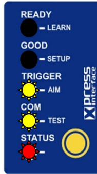
Figure 9 - X-PRESS Interface: Aim Function
