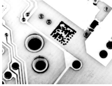
Figure 29 - Data Matrix Code Directly Marked on PCB Surface by Using Laser Etching Technology
