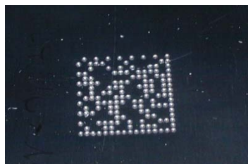
Figure 27 - Directly Marked Dot Matrix Code Characterized by Outstanding Separation Distance between Adjacent Code Elements
