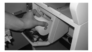
Make sure that a few inches of the paper is extended over the cover edge.  Make sure the paper roll is loaded in the direction as shown in the picture below.
