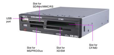
Depending on the customer's requirement, the supported media for the digital media card reader could include all or some of the following:
