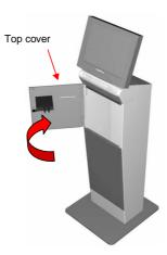
• Lift the middle cover upward before removing it from the casing
