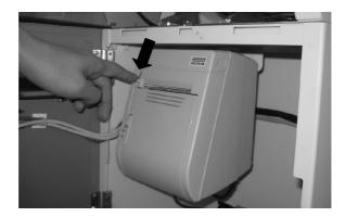
• Remove the spool of the used paper roll from the paper holder and load the new paper roll (as shown in the picture below).
