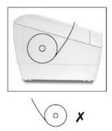
Close the printer cover. Tear the excess paper across the tear bar (see picture below). If necessary, advance the paper by pressing the FEED button.
