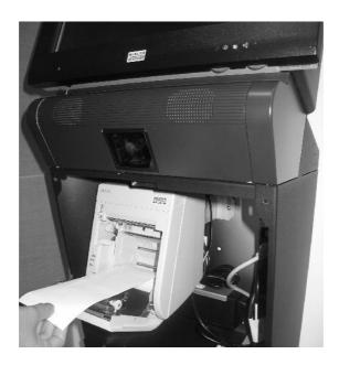
Make sure the paper roll is loaded in the direction as shown in the picture below.
