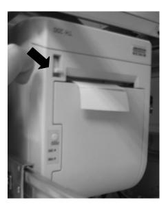
Remove the spool of the used paper roll from the paper holder and load the new paper roll (as shown in the picture below).
