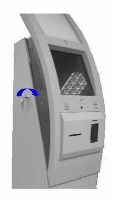
Fully pull out the front bezel in the direction indicated after unlocking the device.
