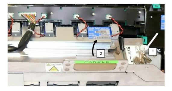
• Remove all hoppers to clean the sensor (1) with a cloth moistened with Isopropylalcohol.
