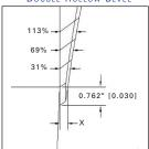
With each regrind, and subsequent new depth adjustment, a thicker blade area becomes exposed to the slit web, causing greater and greater web deformation during slitting. The change of blade width is shown as a percentage of increase from the original width. It is less damaging with the double hollow bevel blade because it is thinner.
