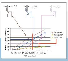
The above graph shows the side load differences for one model top knife holder when the horizontal stroke starting location varies. As can be seen, the closer the blade is to bottom knife, the higher the side load force will be. This is a major factor relative to knife cutting life inconsistencies
