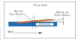
knife edge quickly wears until enough surface area is formed that can support the side force load. Blade dulling begins immediately.
