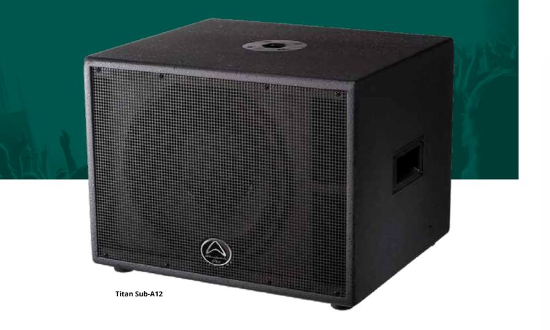
The Titan Sub-A12 is powerful 12" reflex subwoofer designed to provide bass extension for Titan 8A MKII for an incredibly portable sound reinforcement setup. A built-in 250 watt (continuous), 500 watt (peak) amplifier conveniently accepts stereo or mono line level inputs via dual, balanced, XLR-1/4" combo connectors.
