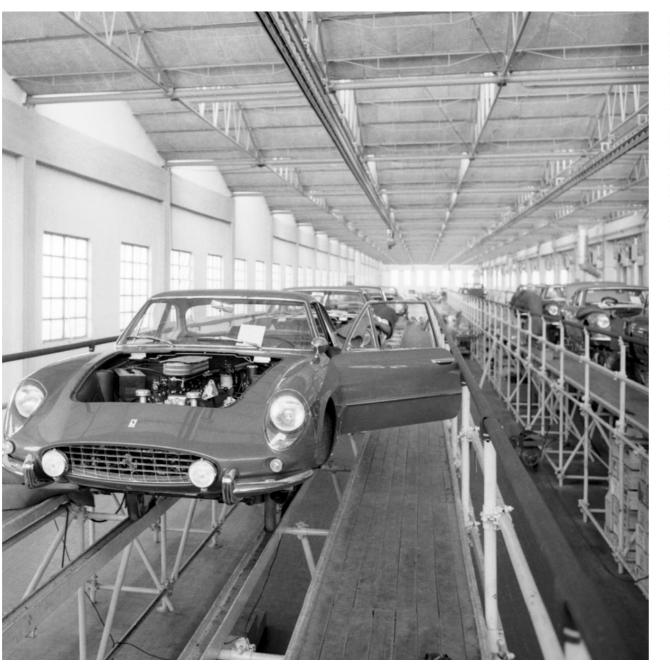
the rear wings. Under that unusually swoopy bonnet was a sophisticated iteration of Ferrari's fabulous V12, now increased to almost four litres in capacity, whose triple Weber carburettors helped it produce 340bhp. These were heady numbers for the period, and represented a major shift for Ferrari, propelling the marque yet further into the stratosphere. For the boutique Italian sports car-maker was now making high-performance luxury cars.
