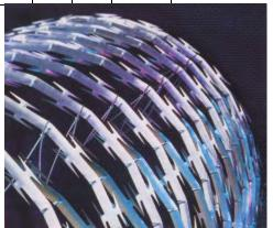
Single coil non-reinforced concertinas 30" in diameter are fabricated from 0.025" thick AISI 301 SS (Stainless Steel). Each roll consists of 101 coil loops with pairs of loops alternately spot welded together at 5 locations around the circumference. Cluster of 4 needle sharp barbs are located 4" o.c. along the spiral turns. Non-reinforced concertinas are only available in stainless steel.
