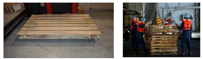
$3990-00-935-7960 - 40 \ge 48$ ", 4 way entry, stringer winged pallet, 1,500 lb capacity  $3990-01-041-8803 - 40 \ge 48$ ", 4 way entry, stringer winged pallet, 3,000 lb capacity  $3990-01-018-6686 = 40 \ge 48$ ", 4 way entry, block winged pallet, 4,000 lb capacity
