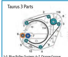
1-5. Blue Pulley System; 6-7. Orange Groove Grommet Assembly, 8. Drive Pulley, 9. Drive Belt, 10. Tension Arm, 13. Foot Assembly Stabilizer
