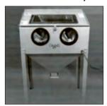
Blasting chamber accepts glass panels as large as 25 x 33". The Sandblast 2533 System includes: 18" deep attached abrasive hopper with trap door, lens protector, a 2-1/2" ferrule for vacuum hook-up, a Model A high velocity blasting gun, 3 medium steel nozzles, and air jet and a light kit - 780 TL
