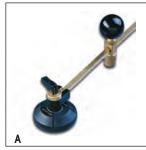
This Silberschnitt® Pro Circle Cutter features a 135° carbide cutting head and a ball bearing swivel action that results in better traction while scoring. The 135° head acts to open the score as it traces making this cutter the best choice for glass 1/16 to 1/4" (2-6mm) thick. Cuts circles from 2-1/2 to 24" wide. Ruled in inches and millimeters, a professional quality tool.
