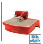
This user-friendly, powerful saw allows you to cut fused art glass and borosilicate glass easily. It will cut a piece of glass up to 1-1/2" thick. The blade cuts in all directions and even grinds as it cuts creating smooth edges. Needs minimal maintenance and is easy to clean up. Additional specifications: belt drive motor, 12-1/2 x 16-1/2" work surface. Included: 5-3/4" standard grit blade, instructional DVD and blade stabilizer.
