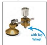
The Circle Supercutter features a single motion vacuum cup and registration marks for accurate alignment and easy attachment to the glass surface. The pivoting, self oiling blade rotates for left or right hand scores and locks onto a ruled, 24" bar for precise adjustment. Uses TOYO's patented Tap Wheel® technology on a 153° angle blade. This cutter is designed to score glass between 1/4" (6.35mm) and 3/4" (19mm) thick. Dropship only.
