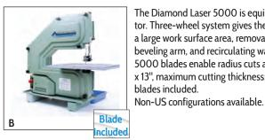
The Diamond Laser 5000 is equipped with a variable speed motor. Three-wheel system gives the saw a 12" throat depth. Includes a large work surface area, removable water tray, a quick-adjusting beveling arm, and recirculating water pump. The Diamond Laser 5000 blades enable radius cuts as tight as 1/2", work surface: 15 x 13", maximum cutting thickness: 3/4", 2 diamond coated steel blades included.
