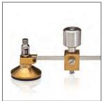
The Toyo Circle Supercutter features a rubber vacuum cup and scribed alignment demarcations for accurate tool placement. The thrust bearing unit is positioned on a pivoting radius bar which is ruled for precise adjustment. The blade rotates 360° to allow for positive tracking along the path of the circle at any radius. The cutting head has a replaceable wheel and axle as well as
