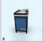
Denver Glass Machinery has developed a diamond grinding system that eliminates the need for several separate grinding wheels. Interchangeable magnetic discs allow the operator to go from rough grind to a final polish with one machine. Obtain true flat surfaces, seam edges and bevel large pieces of glass. Results can be fully controlled by selecting the correct abrasive and the right amount of water with the desired rpm's to achieve the finish that is needed.
