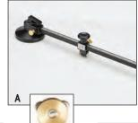
Scores perfect circles from 3 to 28" (76-711mm). Includes straight edge attachment for straight line glass scoring. Secured to glass using a suction cup on cutter base. Max glass thickness of 1/4" (6.35mm). Equipped with a 3 wheel turret. Diameter scale markings in in. and mm.
