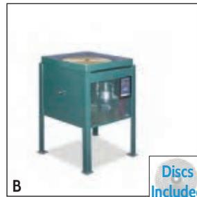
Includes: 1 each - 60 and 260 grit diamond disc, pre-polish 180 blue and 360 brown disc, synthetic felt polishing pad. Pictured with optional brush guard. This system includes a fixed speed machine with a suggested disc set. Available without disc set and/or a variable speed option. Dropship only.
