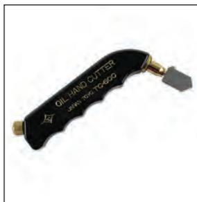
Pistol Grip Straight Cutter is designed to score glass between 1/4" (6.35mm) and 3/4" (19mm) thick using Toyo's Tap Wheel® technology on a 153° angle blade.
