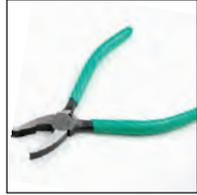
These pliers are a specially designed tool for nibbling or grozing the edge of glass to remove irregular or oversized portions in case the glass was cut incorrectly. One of the pliers' jaws is curved, while one is flat but both are serrated on the inside. Jaws will open to 3/8" wide and pliers measure 6-1/4" overall.
