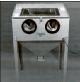
Blasting chamber accepts glass panels as large as 25 x 33". The Sandblast 2533 System includes: 18" deep attached abrasive hopper with trap door, lens protector, a 2-1/2" ferrule for vacuum hook-up, a Model A high velocity blasting gun, 3 medium steel nozzles, and air jet and a light kit - 780 TL
