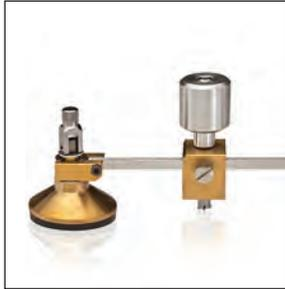
The Toyo Circle Supercutter features a rubber vacuum cup and scribed alignment demarcations for accurate tool placement. The thrust bearing unit is positioned on a pivoting radius bar which is ruled for precise adjustment. The blade rotates 360° to allow for positive tracking along the path of the circle at any radius. The cutting head has a replaceable wheel and axle as well as an automatic lubrication system activated when pressure is applied to the cutting handle. 140° Cutting head.
