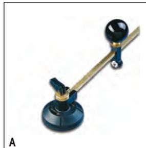
This Silberschnitt® Pro Circle Cutter comes with a six-wheel turret and a heavy-duty suction unit to ensure placement while cutting. The Pro Circle Cutter is calibrated in centimeters and inches. Professional quality tool for cutting glass with a thickness of 1/8 to 1/4" (3 - 6 mm). 130° cutting heads included.
