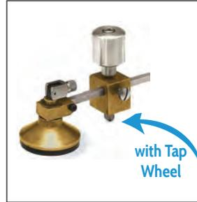
The Circle Supercutter features a single motion vacuum cup and registration marks for accurate alignment and easy attachment to the glass surface. The pivoting, self oiling blade rotates for left or right hand scores and locks onto a ruled, 24" bar for precise adjustment. Uses TOYO's patented Tap Wheel® technology on a 153° angle blade. This cutter is designed to score glass between 1/4" (6.35mm) and 3/4" (19mm) thick. Dropship only.
