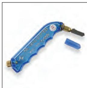
Toyo's patented Tap-Wheel® Technology adds a micro vibration as the wheel rotates, driving scores deeper with less applied pressure. The result is easier breakouts, cleaner edges, less hand fatigue and a longer lasting tool.
