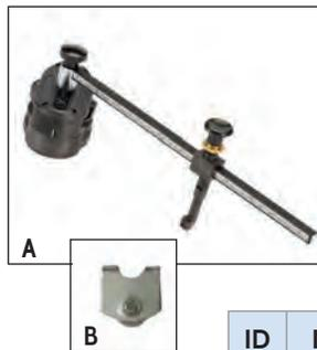
The Fletcher-Terry Oval/Circle Cutter allows you to cut ovals from 4-1/2 x 5-1/2" to 21 x 24" and circles from 4-1/2 to 21" in dia. Equipped with a suction unit, this handy tool ensures secure placement while cutting. Max glass thickness of 1/4" (6.35mm). Uses a 134° carbide wheel. Diameter scale markings in in. and mm.
