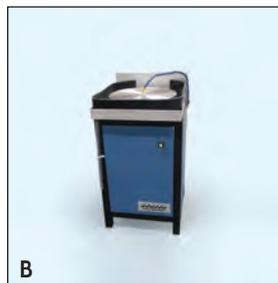
Denver Glass Machinery has developed a diamond grinding system that eliminates the need for several separate grinding wheels. Interchangeable magnetic discs allow the operator to go from rough grind to a final polish with one machine. Obtain true flat surfaces, seam edges and bevel large pieces of glass. Results can be fully controlled by selecting the correct abrasive and the right amount of water with the desired rpm's to achieve the finish that is needed.
