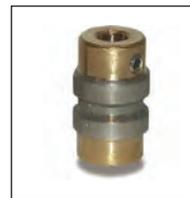
The mirror bit is recommended for decorative mirror edging, mosaic pieces or anytime you want a decorative edge. The profile of the bit will slightly taper the back and front side of your glass piece and the fine grit of the head will leave a soft frosted and smooth (chip-free) edge. Simply position the head so that your glass will pass through the groove in the bit.
