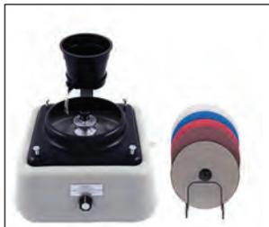
The AmeriTool 8" heavy duty grinding and polishing machine with accessories include: variable speed ball bearing DC motor with 115 VAC converter and coolant reservoir with splash guard; direct drive on 2" flange, 180 mesh metal bond diamond disc, hydraulically pressed to a backing plate; 325, 600, and 1200 mesh sanding discs; white polish pad with 14,000 mesh diamond compound; 4 disc backing plates.
