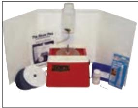
Create your own custom bevels in four easy steps, or reshape and polish stock bevels in just a few minutes. The Studio Beveling System is also great for coldworking fused projects, and includes a Max Grinder base, a 6" diamond disc, 15 and 60 micron grit laps, polishing pad, polishing compound, a Max splash shield with water bottle, and an instructional video. Additional specifications: Shaft: 2-1/8" h x .3" dia., stainless steel.
