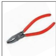
Studio Pro 3/8" Breaker/Grozer Pliers; steel with rubber coated handles. Get double the use out of this handy tool. Use the breaking pliers to break glass along score lines. Turn pliers over and use as grozers to nibble glass away from edges. The spring-loaded jaws work easily.
