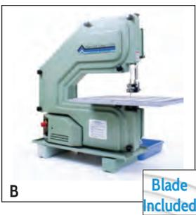
The Diamond Laser 5000 is equipped with a variable speed motor. Three-wheel system gives the saw a 12" throat depth. Includes a large work surface area, removable water tray, a quick-adjusting beveling arm, and recirculating water pump. The Diamond Laser 5000 blades enable radius cuts as tight as 1/2", work surface: 15 x 13", maximum cutting thickness: 3/4", 2 diamond coated steel blades included. Non-US configurations available.
