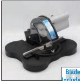
Specially designed to cut zinc, brass, copper, and steel. Cuts up to 3/4" thick material. Adjusts for cuts from 45-90° in either direction. Features a bolt clamp to hold came in place while cutting. Complete with ultra thin "abrasive" blade which cuts cleanly and quickly.
