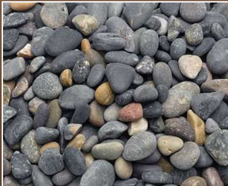
Well-rounded, spheroidal grains
