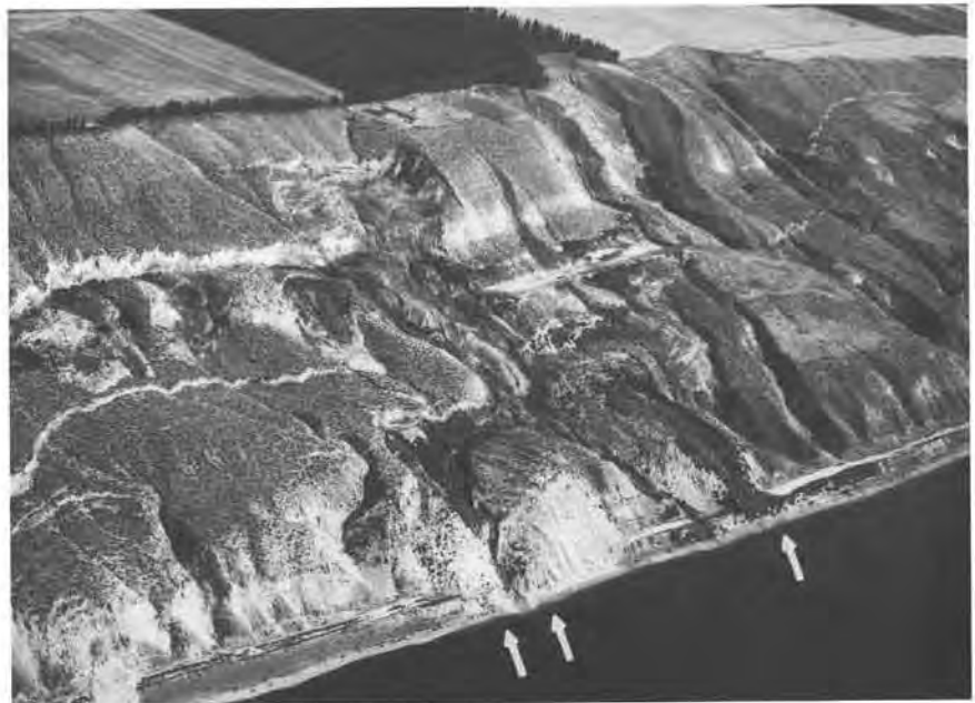
Figure 13. Landslides that blocked a county road along the Columbia River in 1979 (double arrow) and 1981 (single arrow) at the north end of the Johnson Island landslide area. Bluffs in the photo average 160 m high. Photograph was taken in 1983; view is to the southeast.
