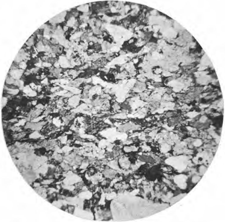
FIGURE 2. Photomicrograph of graywacke of the Chilliwack Group. Angular to subangular fragments of chert, quartz, plagioclase, and rock chips. Practically no matrix present. ( \times 15 —plain light.)
