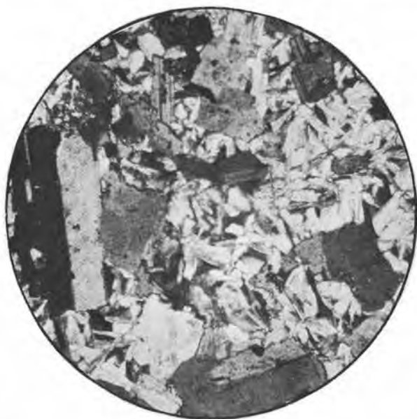
FIGURE 21. Photomicrograph of quartz diorite of the crystalline complex. Quartz, plagioclase, and orthoclase with interstitial prehnite. Prehnite forms divergent crystals. ( \times 60 —crossed nicols.)
