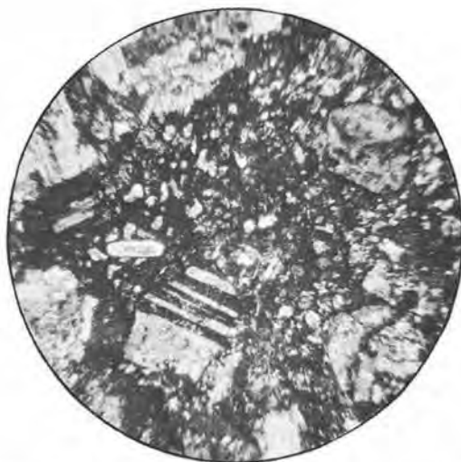
FIGURE 14. Photomicrograph of andesite tuff. Twinned plagioclase crystals surrounded by fragments of andesite, plagioclase, and volcanic glass. ( \times 15 —crossed nicols.)
