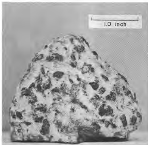
FIGURE 15. Saxonite from the Sumas Mountain Serpentinite. Unaltered enstatite crystals (dark gray) surrounded by serpentinized olivine (light gray).
