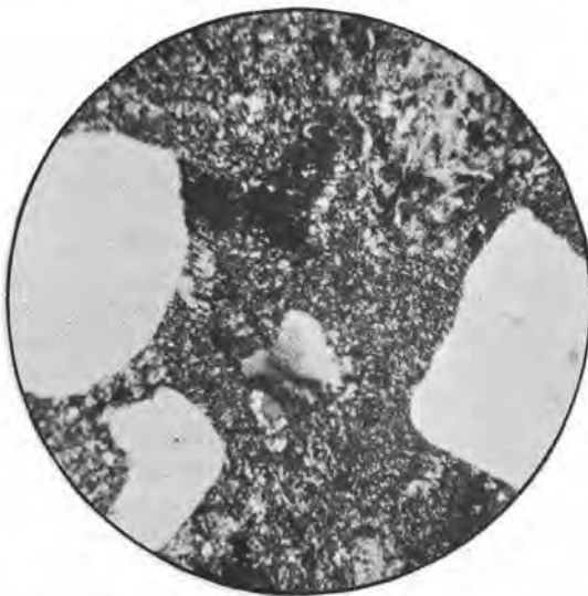
FIGURE 12. Photomicrograph of porphyritic dacite. Chert-like groundmass of quartz and feldspar surrounds rounded phenocrysts of quartz. ( \times 63 —crossed nuclei.)
