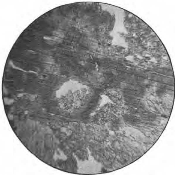
FIGURE 24. Photomicrograph of porphyroblastic diopsidite of the crystalline complex. Hornblende (dark gray) partially replaced by diopside (medium gray). ( \times 33 —plain light.)
