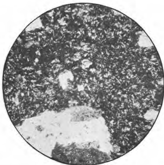
FIGURE 9. Photomicrograph of porphyritic andesite. Plagioclase ( An_{20} ) phenocrysts surrounded by chlorite, augite, and saussuritized plagioclase. ( \times 60 —crossed nicols.)
