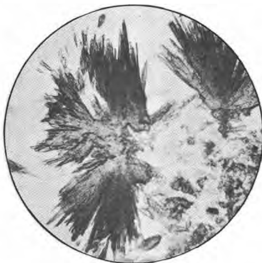
FIGURE 10. Photomicrograph of pumpellyite in greenstone. Pumpellyite (dark-gray radiating needles) in albite (white). ( \times 90 —crossed nicols.)
