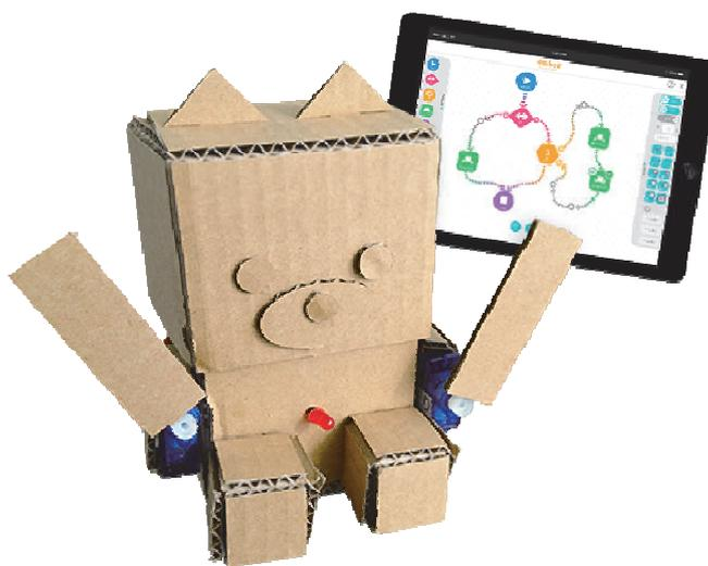
Photo 2 The “embot” robot for teaching programming
