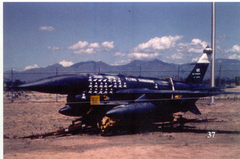
The FLYING SUBMARINE was a Ryan AQM-3Q target drone that was launched by a DC-130. After each sortie, the drone was painted with a White mission marking on the side. Out of the twenty-three sorties shown, the aircraft went into the water (markings without parachutes) five different times, earning it the name it carried on the fuselage in White. (Author)
