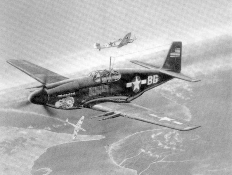
A P-51 Mustang of the 111th Tactical Reconnaissance Squadron (Snoopers), 68th Tactical Reconnaissance Group in Algeria during the Fall of 1943 used an "eyeball" marking on the side of the fuselage to indicate each photo reconnaissance mission flown. The Yellow bands on the wing were recognition markings to help identify the Mustang to friendly crews.
