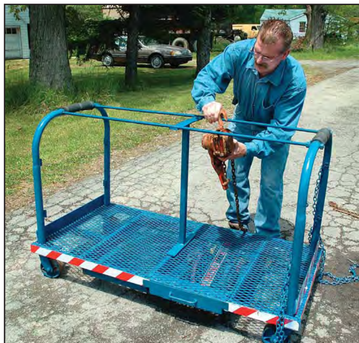
Carl Croscio demonstrates the "Croscio Services Cart," for which he received a patent last month. The cart contains drawers for hand tools and places to hang heavier equipment, such as chain hoists and come-alongs.
