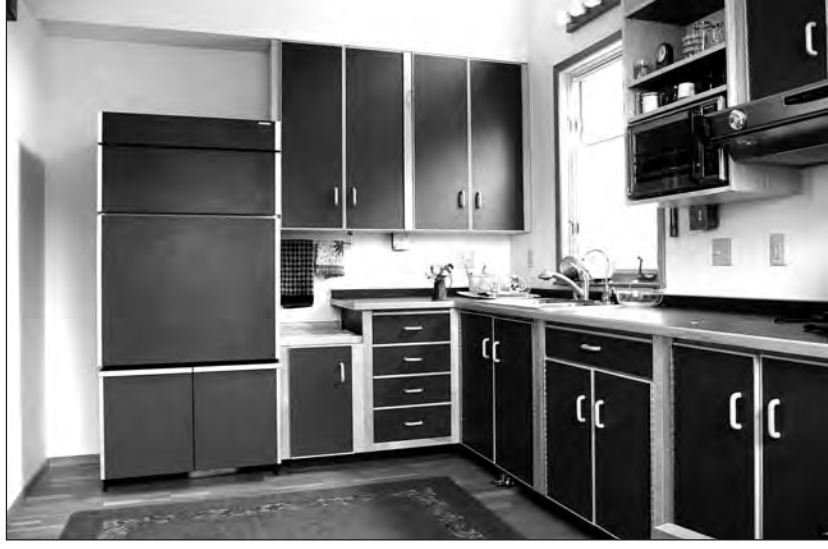
This is one of the most efficient refrigerator/freezers made. Its angular, yet contemporary, appearance allows for high levels of insulation in the walls.
