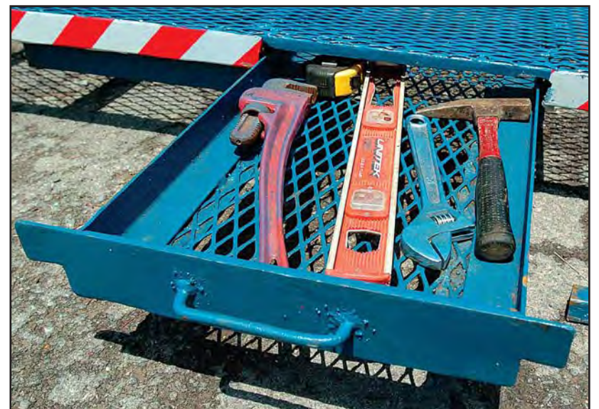
Carl Croscio demonstrates the "Croscio Services Cart," for which he received a patent last month. The cart contains drawers for hand tools and places to hang heavier equipment, such as chain hoists and come-alongs.
